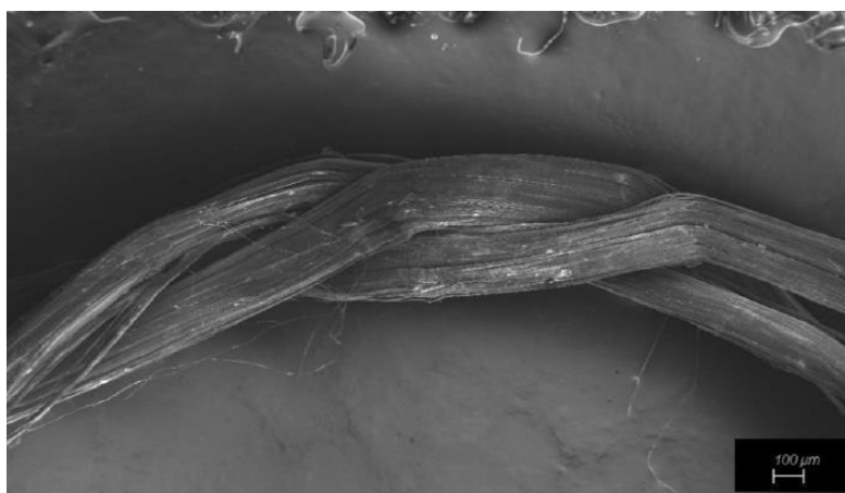
Figure 1: A CNT yarn, 130 \mu m diameter, exploited for the fabrication of a supercapacitor electrode.
